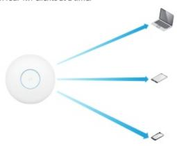
MU-MIMO with 2x2 and 1x1 clients: The UniFi HD AP communicates with one 2x2 client and two 1x1 clients at a time.
