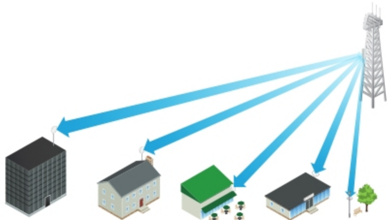
The PowerBeam ac ISO used as a CPE device for each client in an airMAX PtMP network.
