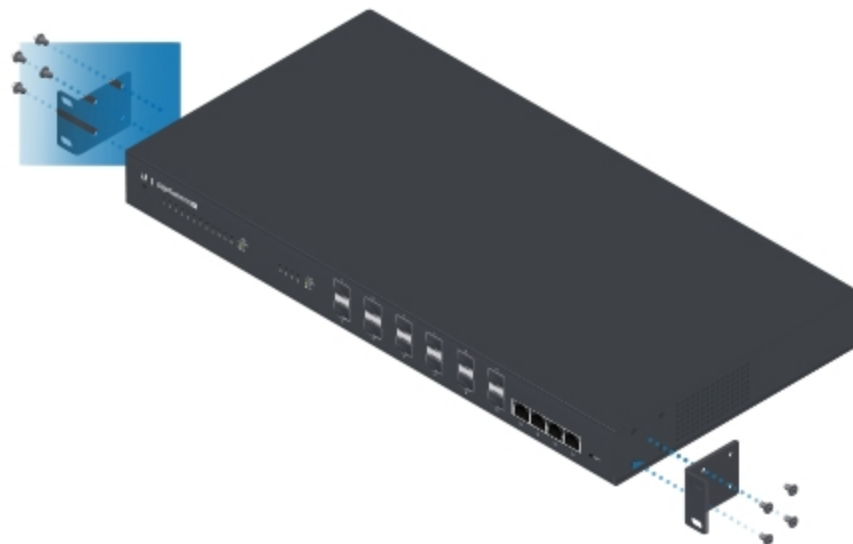
Attaching Rack-Mount Brackets to the EdgeSwitch XG
